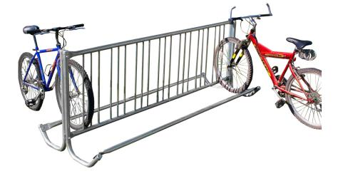
The Modern Double-Sided Bike Rack by UltraSite is a large capacity bike rack that is portable. The frame of the rack is made using 1 5/8" zinc tubing. The rungs in the center of the rack that keep bike tires in place are 5/8". The entire rack is made with a galvanized finish. Heavy duty casted clamps and zinc plated hardware ensure that this bike rack will be a lasting addition to your area. The Modern Double-Sided Bike Rack is available in 5, 8, and 10 foot lengths.
